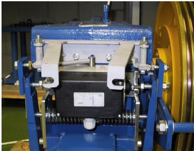
Fig. 6: Remote linkage for remotely opening the Brake Levers.
